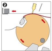
The squeegee moves down and printing starts at the top of the cylinder. The screen frame moves and the vacuum cylinder rotates.
