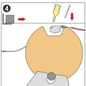
The screen frame starts moving back. The flo-coater starts moving down onto the screen when the squeegee lifts up. The cylinder, keeps rotating for printing the next substrate.
